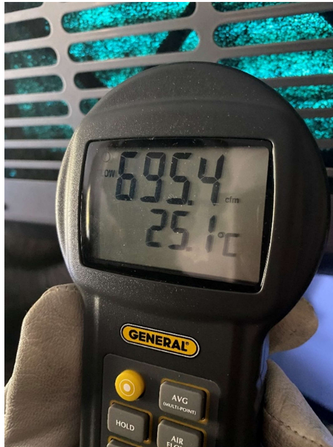
Measured with a General Tools LCD Digital Anemometer Model DCFM700.
